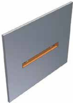
Positioning at the same level to the wall
