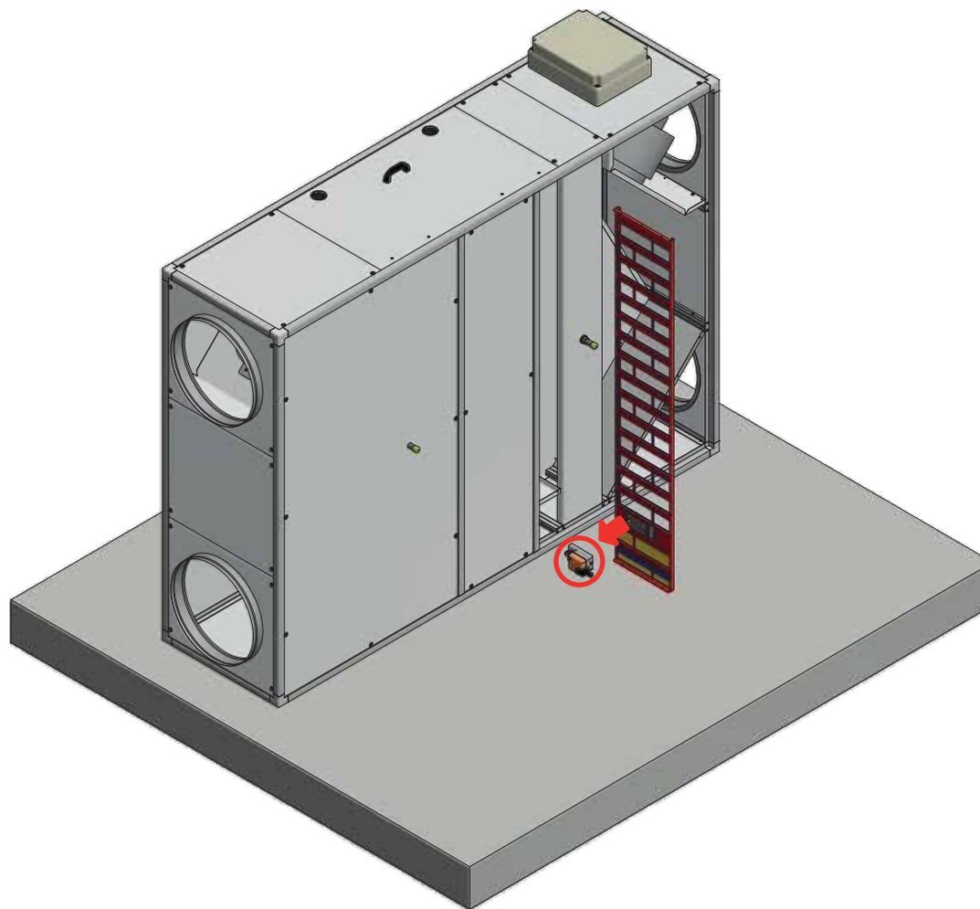
ISTRUZIONI SMONTAGGIO MOTORE BATTERIA / INSTRUCTIONS REMOVING BATTERY
