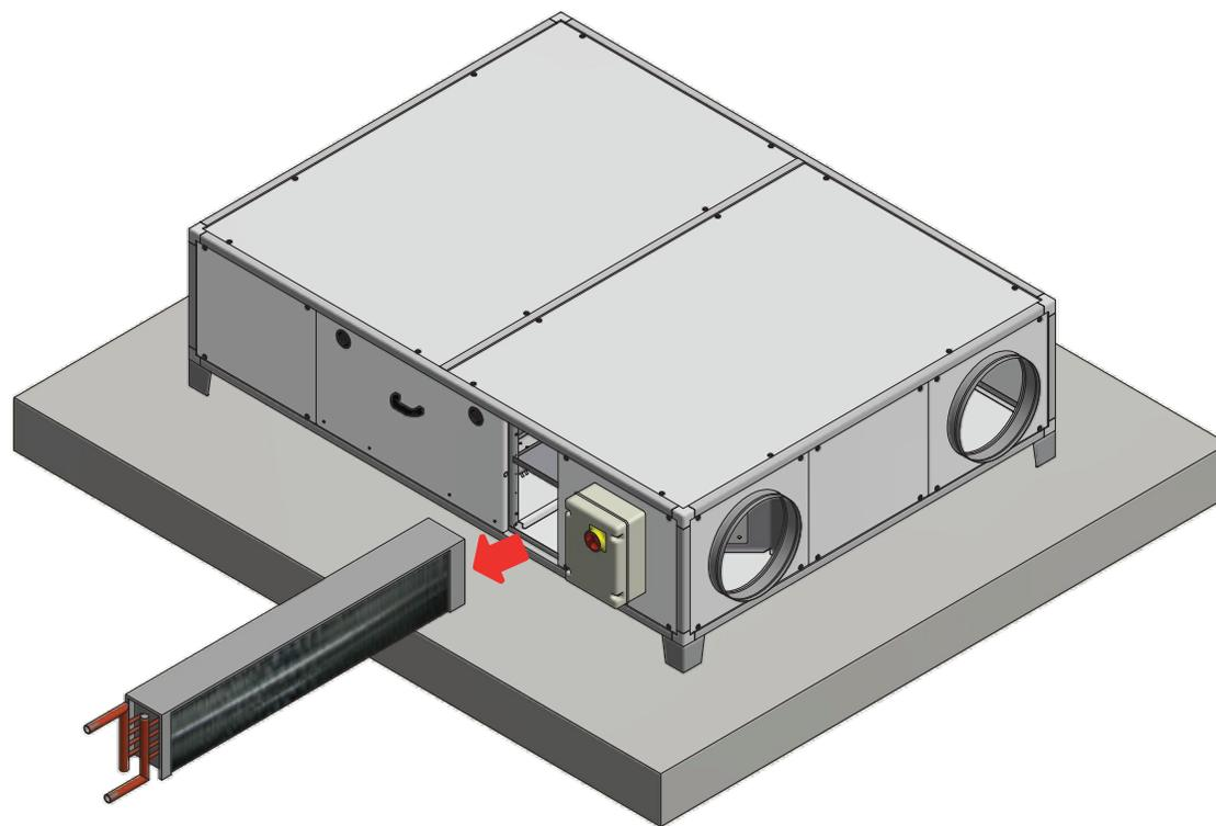
ISTRUZIONI SMONTAGGIO RESISTENZA / INSTRUCTIONS REMOVING RESISTANCE
