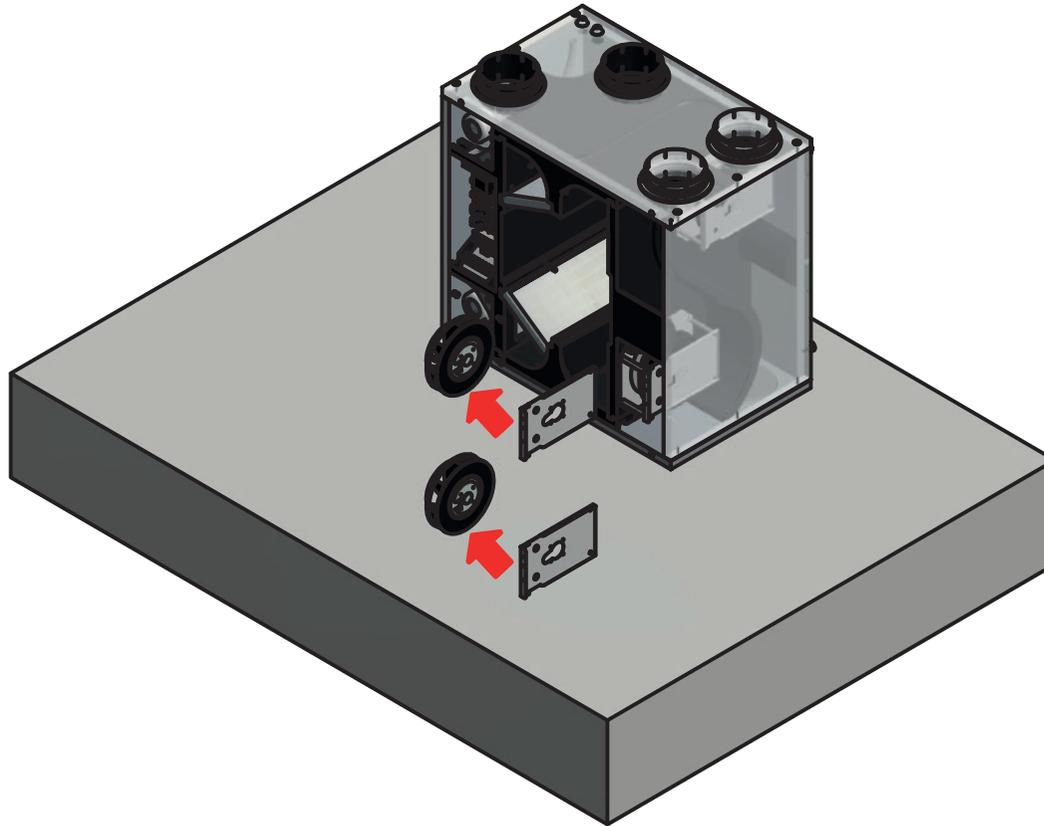
ISTRUZIONI SMONTAGGIO QUADRO ELETTRICO / INSTRUCTIONS REMOVING ELECTRICAL PANEL
