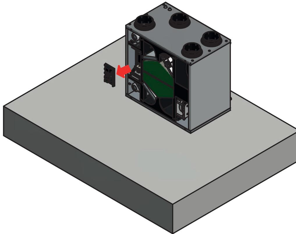
ISTRUZIONI SMONTAGGIO MOTORE BY-PASS / INSTRUCTIONS REMOVING MOTOR BY-PASS
