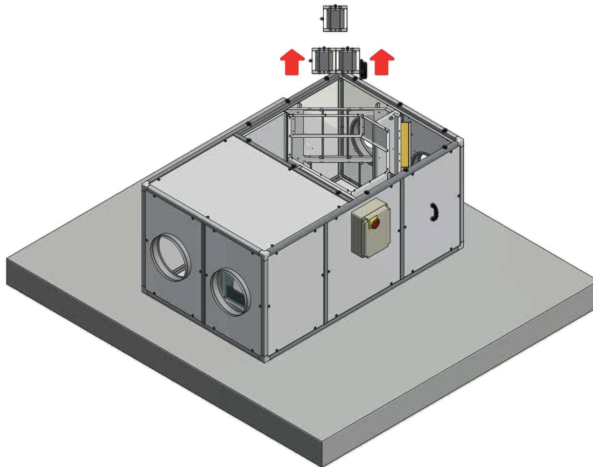
ISTRUZIONI SMONTAGGIO RESISTENZA DI POST RISCALDAMENTO / INSTRUCTIONS REMOVING POST HEATING RESISTANCE
