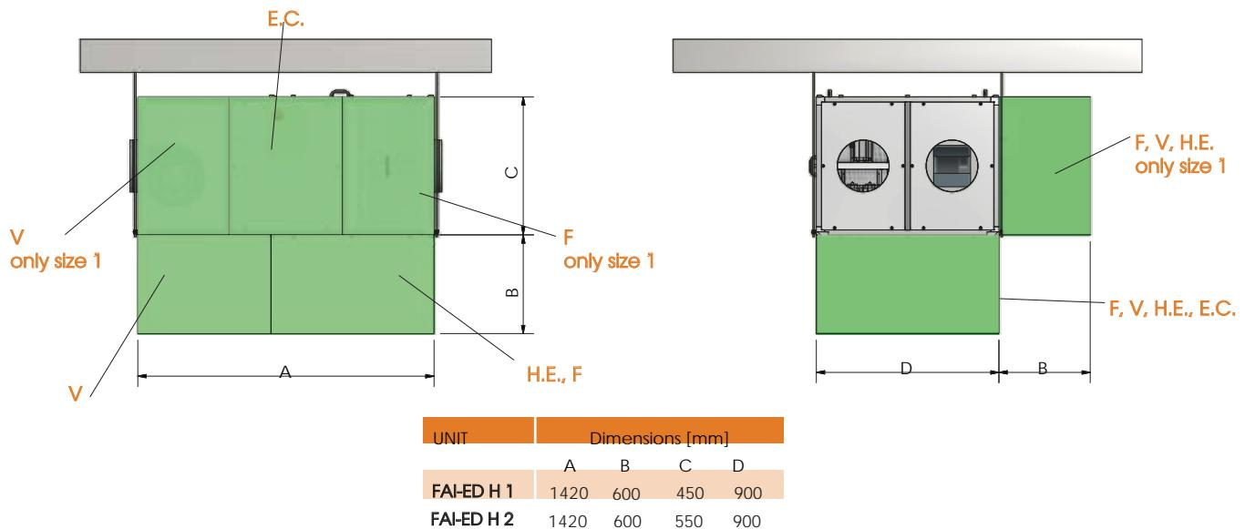
The ceiling installation for 3-4-5 size of FAI-ED H it is not recommended. The manufacturer is not responsible for injury to persons or damages to things in case of this type of installation. **CAUTION:** The operations of inspection of the heat exchanger for these sizes can not be made manually for the high weight of the same which would result in an unacceptable level of risk.
