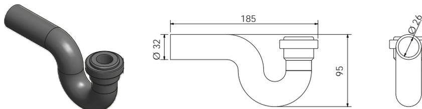
N.B.: predict 1 additional siphon if there is the cold water coil BA-AF / AC or DX gas (duct)
