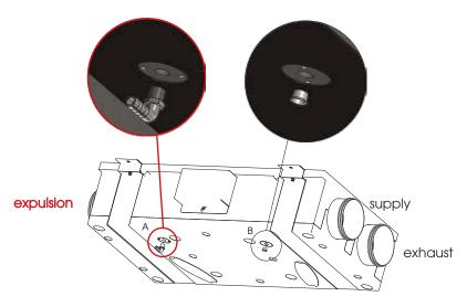
The condensate drain must be mounted near the EXPULSION; N.B. - provide a siphon on the condensate drain circuit
