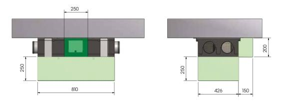
CONDENSATE DISCHARGE ASSEMBLY (90 ° bend hose connection supplied)
