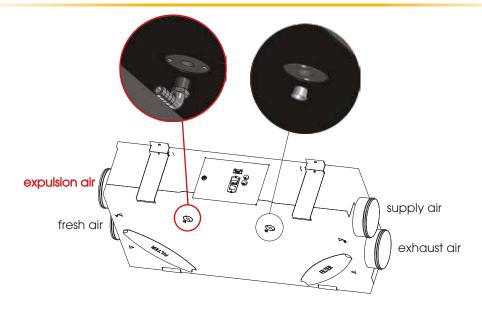
The condensate drain must be mounted near the EXPULSION; provide a siphon on the condensate drain circuit
